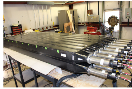
Figure 13: The detector array geometry used in the first LANSCE experiment, consisting of 16 MoNA detectors arranged in two horizontal layers of 8 detectors each. The neutron beam entered the room through a 3-mm collimator, visible in the upper right corner of the picture, and impinged on the array at the center point of the first upper layer detector.
