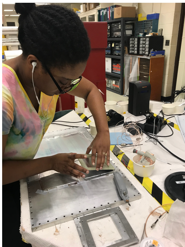
Figure 30: Undergraduate April Christopher working on a prototype GEM detector for next generation MoNA detectors.
